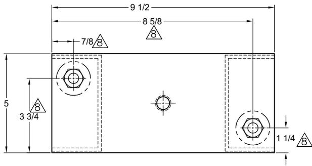
**TYPE ME-2E SPRING ISOLATORS WITH INTERNAL ADJUSTMENT**
